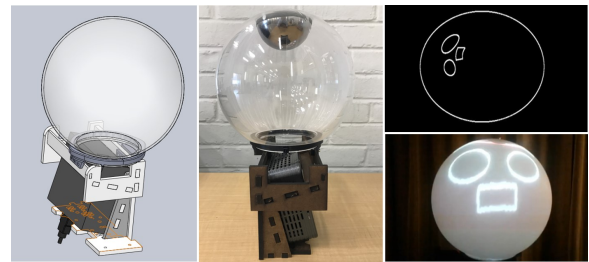
Figure 3: Quori's head hardware CAD (left) and finished head module (middle). Sample warped image to be sent to the projector (top-right) and the final product displayed on the sphere (bottom-right).
